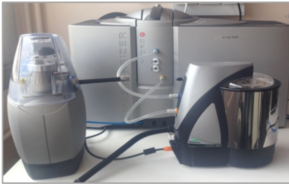
Particle size distribution Liquid or dry phase determined by laser diffraction – Malvern 3000E
